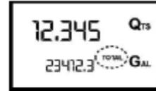
After pressing the RESET key, during reset, the display screen first of all shows all the lit-up digits and then all the digits that are not lit up.
