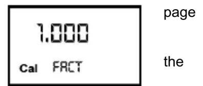
If you are using k24 with “factory k factor”, the display page shown in diagram will be displayed, with the word “fact”.
