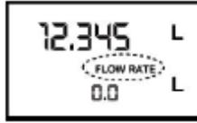
to show a Flow Rate of 0.0 as indicated in the illustration then quickly press RESET.
