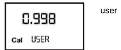
If one “user k factor” has been set, the calibration factor set by the (in our example 0.998) will be displayed. The word “user” indicates a calibration factor set by the user is being used.
