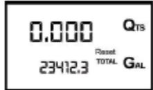
and, after a few moments, the Reset Total is replaced by the NON resettable Total (Total).
